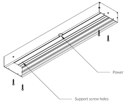
Mount the canopy to the ceiling and connect the power.
