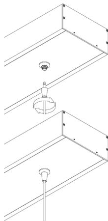
Insert the connector in the hole and screw the cap until the pendant is firmly secured (ensure correct polarity).
