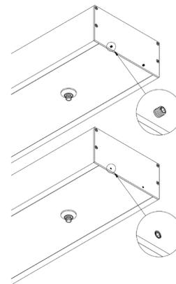
Tighten the side screws until they are flush with the end caps.
