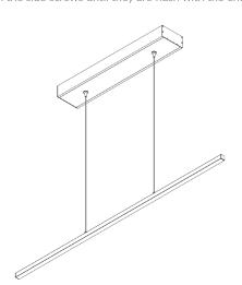
Insert the connector in the hole and screw the cap until the pendant is firmly secured (ensure correct polarity).
