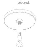
Put on the canopy, and screw the wide cone until the canopy is firmly
