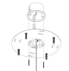
Connect the wires to the power and mount the crossbar to the junction box.
