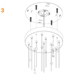
Push the canopy on, and screw the end caps onto the nipples until the canopy is firmly secured.
