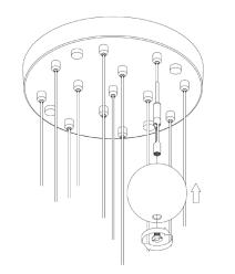
Slide the glass onto the hardware and screw on the end caps.
